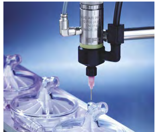
752V dispensing uv-cure adhesive on medical pump.
