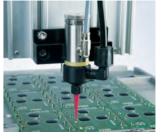
752V valve on robot dispensing on PCB.
