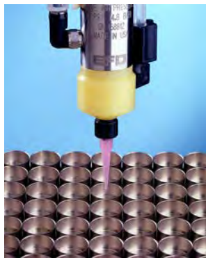
752V filling cans with electrolytes.
